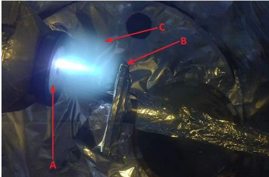
Figure 18: Pulsed laser deposition of TiN from [53]
