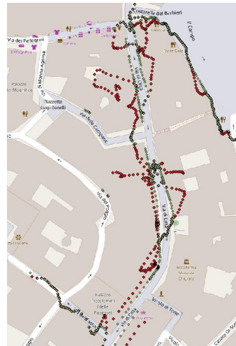
(b) Raw (red points) and GNSS-corrected (green points) data comparison from Siena's urban canyon.
