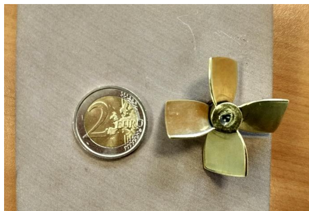
Figure 3.33 4 cm symmetric wind turbine
