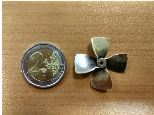
Figure 3.35 3 cm airfoil wind turbine
