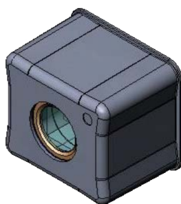
Figure 2.13: STMicroelectronics VW6558 camera module. The casing encapsulates the sensor and a stack of lenses above it.
