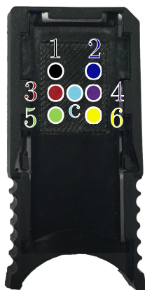
Figure 3.7: Labels for the seven acquisition points on the 3D-printed chip. Each one is associated to a color that is used to plot the acquired spectra in the following figures.
