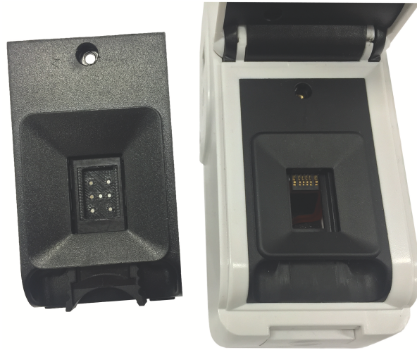
Figure 3.1: CCC with the modified holder next to an unmodified Q3-Plus.
