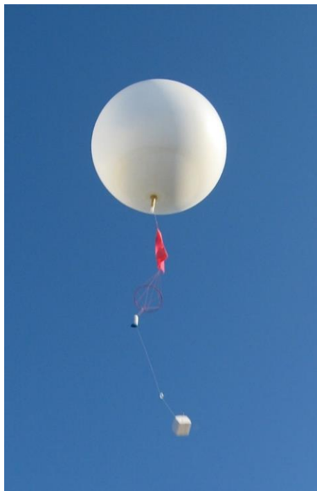
Figure 2.3.1: Typical weather balloon during a flight
