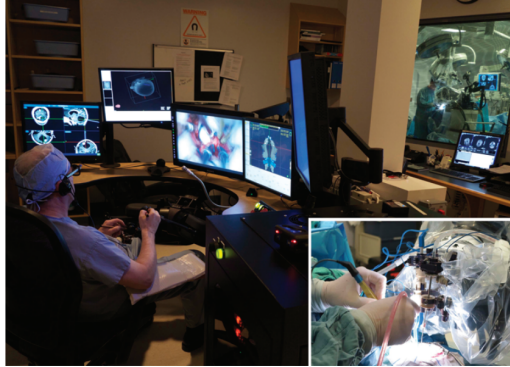
Figure 2.5: The NeuroArm system during a surgical intervention in the operating room. The main picture depicts the workstation where the surgeon commands the haptic hand controllers. The inset displays the neuroArm manipulators and the assistant surgeon while resecting the tumor.
