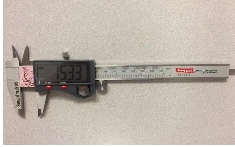
Figure 3.29: The digital caliper with a resolution of 0.01 mm used to measure the size of the rectangular printed patterns.
