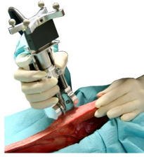
Figure 2.9: The Craniostar, an active robotic wheeled tool for surgical craniotomy, is shown.
