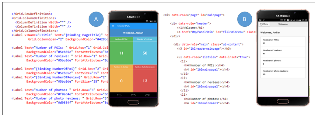
Figure 6.1: Same GUI implementation of our main page in Xamarin(A) and PhoneGap(B).
