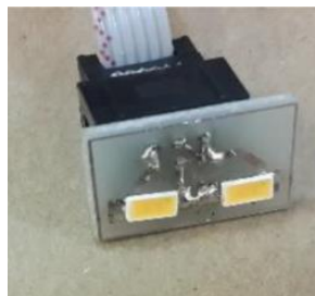
Figure 20 Osram 1Watt LED Test Board
