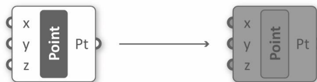
Fig. 30. Schematic representation of a component for point construction (on the left); the same component as switched off and consequently unable to store and transmit any datum (on the right) (elaboration from Tedeschi, 2014).
