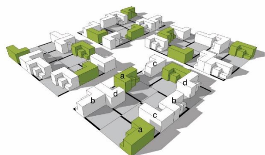
Fig. 102. Identical urban blocks composed from 4 different types of plots with identical building bulks (ibid.).
