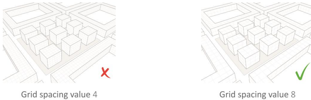
Fig. 117. Extraction of two hypotheses of grid resolution for detailing energy analysis. DIVA 's parameter quantifies the “texture” or the grain of simulated sensors upon the set of imported faces: the smaller the number, the finer the grain, the sharper the computational strain. Having a demanding process of optimization on sight, this latter reason suggested a coarser grid (source: author).
