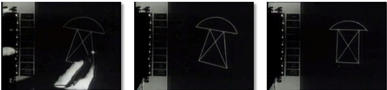
Fig. 60. A process of self-adjustment, starting from manual tracing by light pen, which provided input geometries, and heading automatically to a right-angled version, in conformity with the related constraint expression (retrieved from: http://www.madlab.cc/ ).
