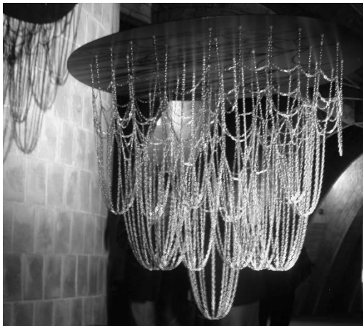
Fig. 48. Two instances of the hanging chain model : on the left, the reconstruction of a battery of catenary curves attached to a plate; on the right, an rigidified and inverted catenary, resulting in a group of optimized arches for specific widths, lengths and weights (retrieved from: https://it.pinterest.com/ ).
