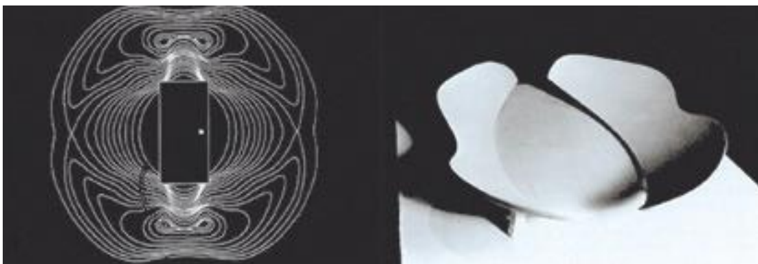
Fig. 51. One of Moretti’s models of stadium, exhibited at the 1960 “ Parametric Architecture ” exhibition at the Twelfth Milan Triennial. On the left, the plan with its corresponding curves; on the right, the resulting three-dimensional model (retrieved from: http://marcolucci.altervista.org/ ).
