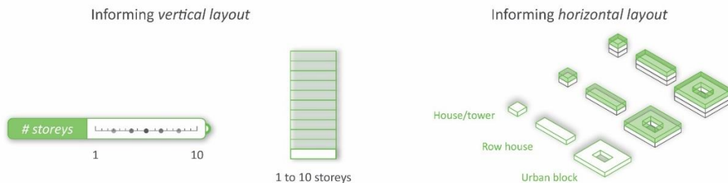
Fig. 89. The two inputs, one for vertical and one for horizontal layout. Vertical layout is informed through a parameter governing the number of generated floors, which is applied to all units; horizontal layout can be distinguished with different input curves, one per each typology (source: author).
