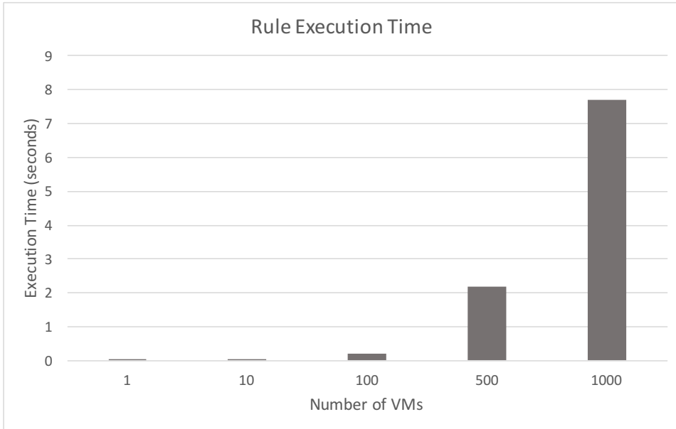
Figure 7.4: Average rule execution time of a single monitoring rule with an increasing number of monitored virtual machines
