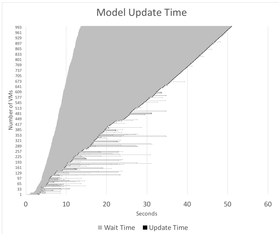
Figure 7.1: Model update time in seconds after starting one thousand virtual machines
