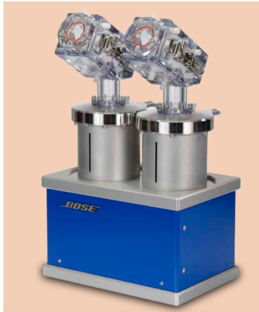
Figure 6.34 The Bose ® DuraPulse ™ used to perform accelerated fatigue test.
