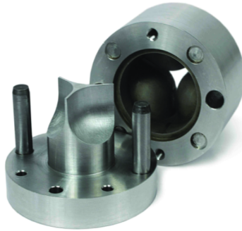
Figure 4.14 Mould used to manufacture PHVs by compression moulding
