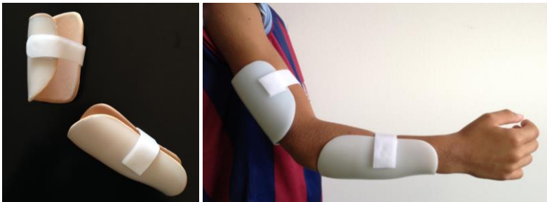
Figure 3.5 The figure on the left displays a personalised set of shells built for a healthy subject to validate the entire acquisition plus CAD-aided limb modelling procedure; the prototype fits perfectly on the subject's limb even without the necessity to add padding inside the valves, as shown on the right . The padding is employed to increase the comfort softening the interface between the soft skin and the rigid valve and to add secure pinching grip.
