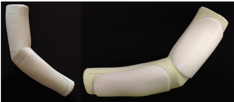
Figure 3.13 The figure displays, on the left , the physical model of the arm shaped by the CNC machine (7-axis mill) from a polyurethane foam. On the right , the polypropylene shells formed under vacuum using the model as a positive mould and cut following the biomechanical design.
