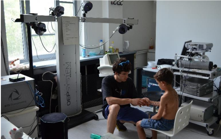
Figure 3.4 Set-up for the limb surface acquisition. The optoelectronic system uses 8 infrared cameras. During the acquisition, the subject is free to move inside the FOV. By holding the subject's finger, the researcher gently controls any exceptional involuntary movements, favouring the optimal posture (close to a neutral arm habit), maximising marker visibility.
