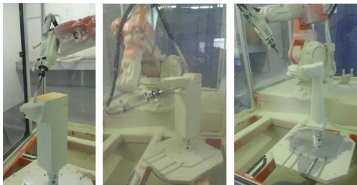
Figure 3.8 The CNC machine in action: a 7-axis mill shapes the polyurethane foam block to obtain the positive limb model based on the virtual reconstruction from the point cloud converted into stereolithographic .stl format.
