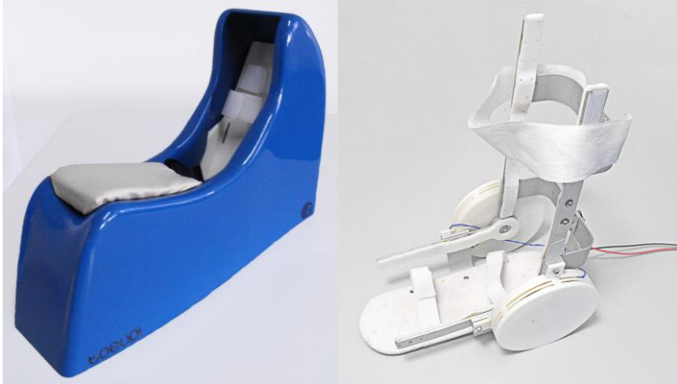
Figure 2.12 Two examples of active devices used for the neurorehabilitation designed by CNR-ICMATE. Both the mobilisers are activated exploiting the shape-memory effect. It is worth to notice that Toe-UP! mobiliser ( left ) can be used by neurological patients in the early stages of their recovery process and it is provided with a NiTi-based linear actuator; on the right , the ankle mobiliser Leia is equipped with two patented rotary actuators including NiTi wires, and its special design aimed at reducing electromagnetic emissions allows its use in very sensitive and strictly-ruled environments, such as MEG or MRI.
