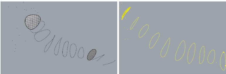
Figure 3.6 The figure shows the first step in the process to create the virtual arm model from the point cloud collected with the optoelectronic system. From the point cloud, each ring, that defines the contour of the limb, is reconstructed by interpolating with a 3 rd -order spline the points that belong to the same circle of markers, or limb slice.
