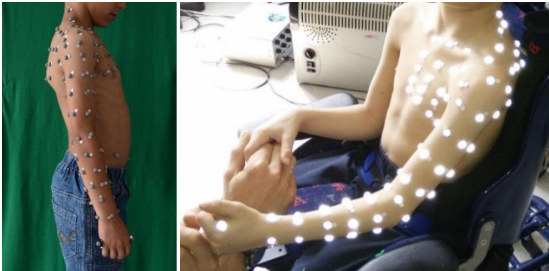
Figure 3.9 The figure shows markers positioned on the skin. The 105 reflective passive markers are positioned with a repeatable and defined scheme to obtain a structured points cloud, easier to replicate for every subject. On the left is depicted a healthy subject standing in the FOV; the acquisition of markers takes only a few seconds. On the right is shown the same marker placement for a dyskinetic subject. In this case, during the acquisition, even if the patient is left free to move in the FOV, the operator helps him stabilise posture to achieve the best arm positioning, by gently holding his fingers.
