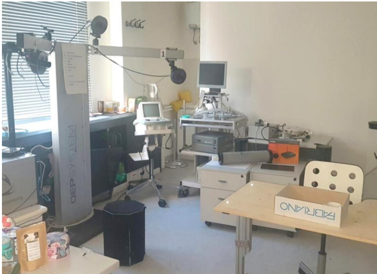
Figure 4.2 The photo shows the laboratory where the acquisitions were carried out. In particular, the BTS SMART-Elite System with 8 infrared cameras that has been used to acquire the motion of the upper limb, the table and the adjustable-in-height chair at the LARES laboratory (Laboratory of Analysis of the Breath located in the Department of Electronics, Information and Bioengineering of the Politecnico di Milano, Milan – Italy).
