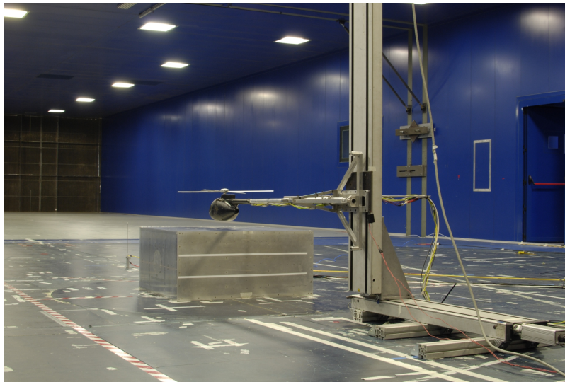
Figure 2.7: The rotor-obstacle test rig mounted inside the GVPM wind tunnel
