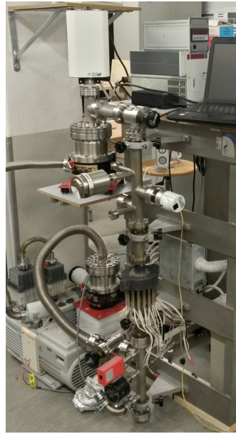
Figure 3.12: PERI II facility in vertical position. Upper part is the low pressure section keeping constantly at pressure in the range of low 10^{-4} Pa. Here a quadrupole mass spectrometer detect the hydrogen concentration during the time. The bottom part is the high pressure section. After a vacuum in order of 10^{-4} Pa is filled by pure hydrogen. In this work a partial pressure of 100mBar is used.
