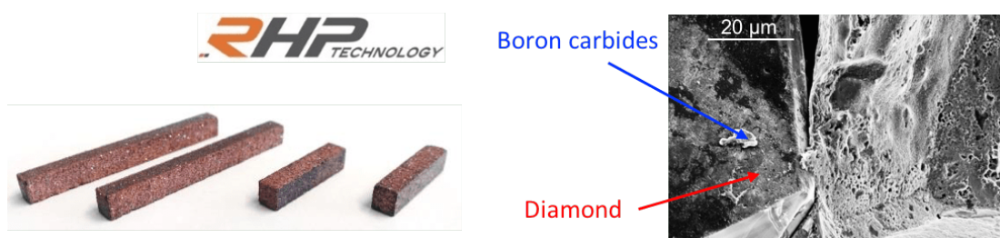
Figure 4.11: \text{CuCD} samples (left) and high magnification SEM observation on a fracture surface of \text{CuCD} (right). Courtesy of N. Mariani, CERN.
