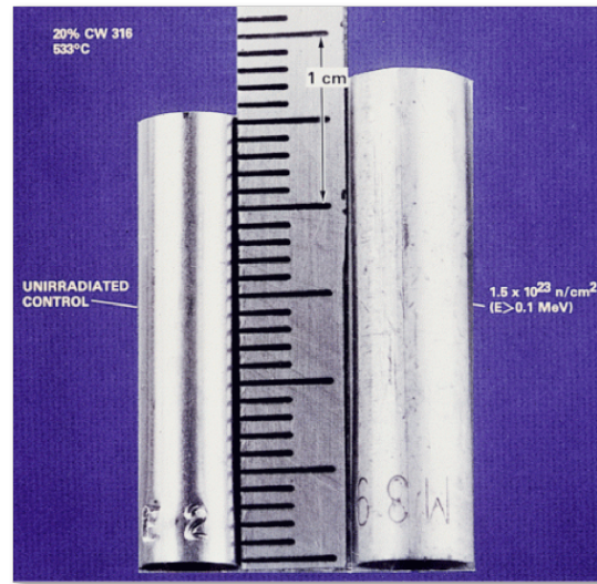
Figure 1.8: Void swelling in 316-stainless steel tube exposed to reactor dose of 1.5 \times 10^{23} \text{ n/cm}^2 : (left) before irradiation, (right) after irradiation. Picture from Ref. [38].
