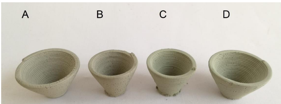
Figure 73. 3D-printed empty truncated cones: A geopolymer at 55°; B geopolymer at 65°; C microalgae at 65°; D microalgae at 55°.
