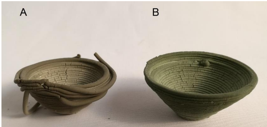
Figure 72. 3D-printed empty truncated cones at 45° of inclination: A geopolymer; B with microalgae.
