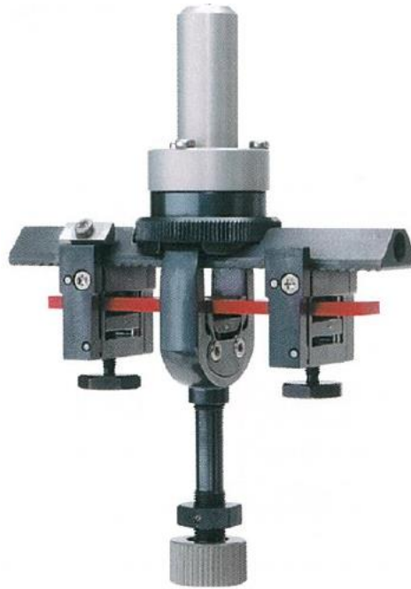
Figure 26. Example of three-point bending configuration [79].
