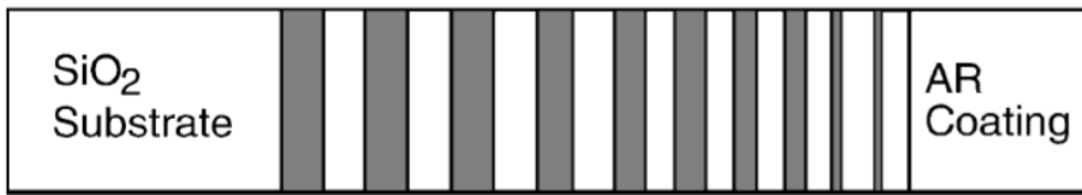
Figure 1.16: Schematic picture of the universal structure of a double-chirped mirror. AR, anti-reflection. Copyright [27].
