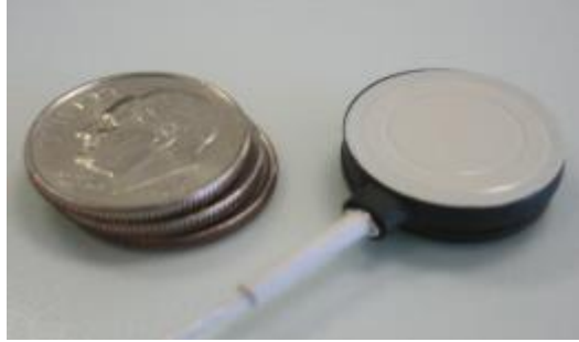
Figure 2.5: QUASAR capacitive biosensor with 10c coins for scale [12]
