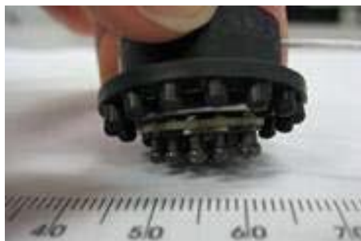
Figure 2.4: QUASAR hybrid EEG biosensor [12]
