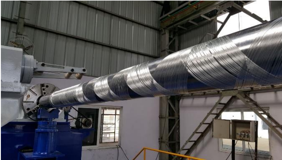
Figure 37 - Filament winding of a composite pipe with \pm 55^\circ [deg] winding-angle [35]
