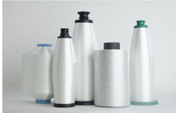
Figure 9 - Yarn of glass fibres [33]
