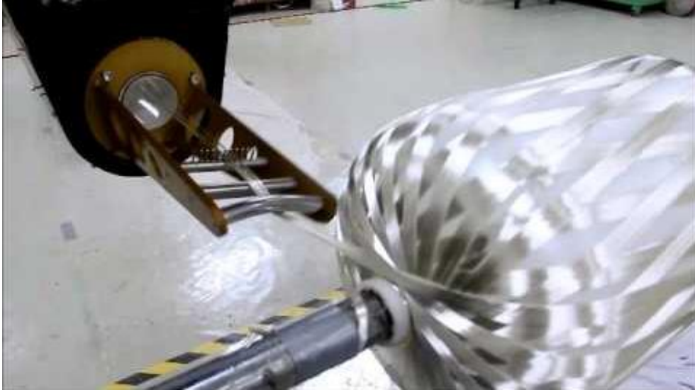
Figure 42 - Deposition head of a 5 degrees of freedom filament-winding machine [34]
