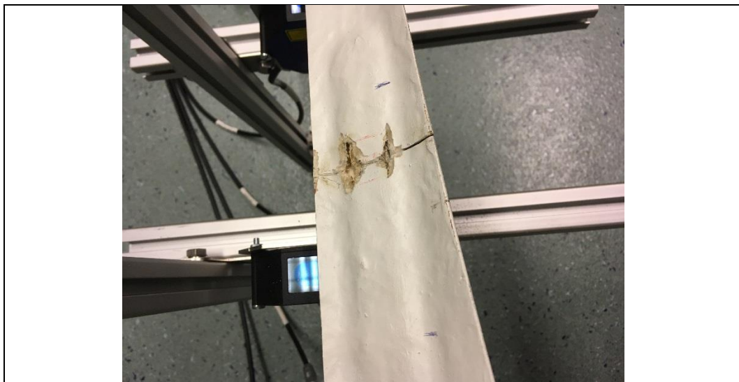
Fig. 3-39 Blade model with one crack
