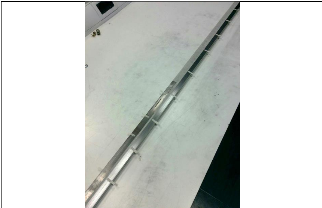
Fig. 2-29 Beam attached with fiber optic
