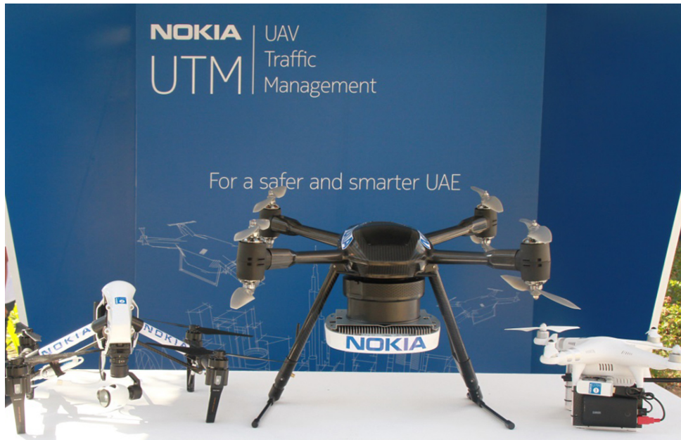
Figure 1: An example of an aerial base station quadcopter from NOKIA working at 4G
