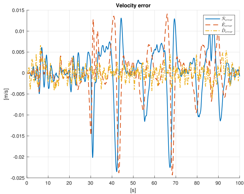
Figure 4.12: Geometric control with modified attitude reference: velocity error in eight-shape trajectory simulation with measurement noise
