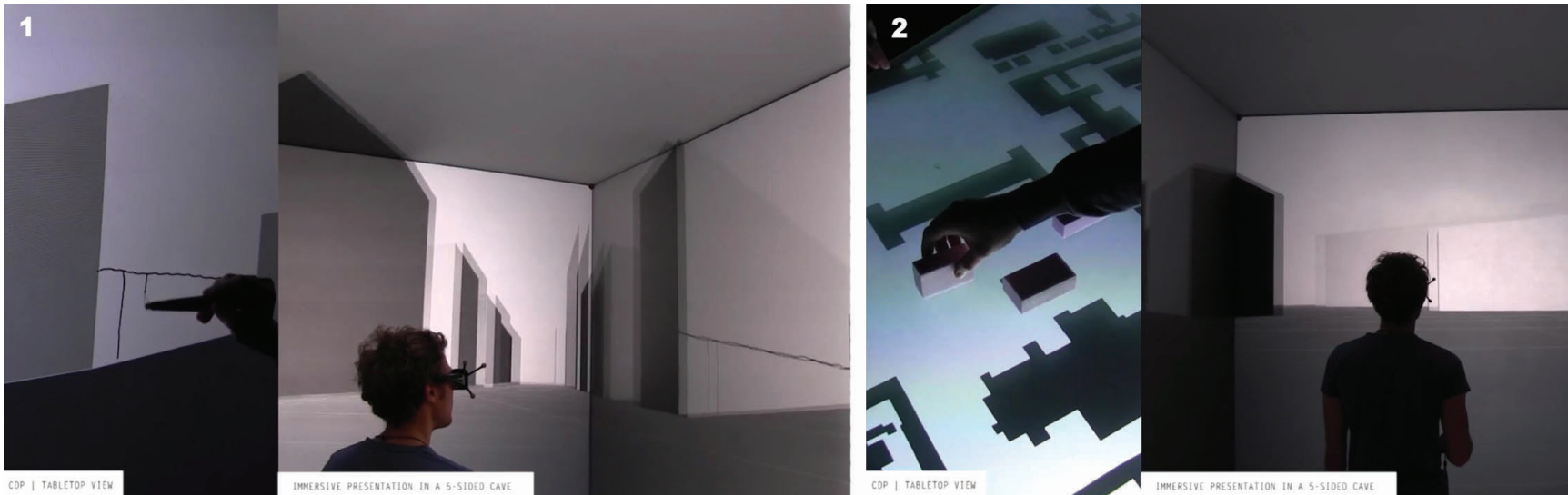
Fig 2.11 | Screenshot's video "From Physical to Digital" | 1- interactive sketches: freehand drawing on device visualized inside immersive environment at the same time; 2- from physical to virtual: change immersive environment moving maquette elements on luminous planning table ( https://vimeo.com/79087334 )
