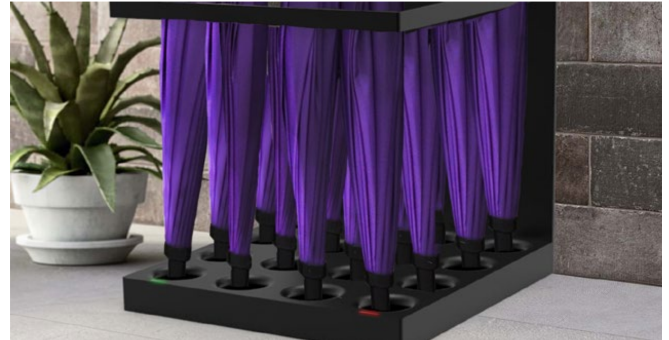
Fig 6.2 Umbrella stand details. Green light mean unlocked, red light means booked and no light means that the umbrella is available to be booked. Source: The author
