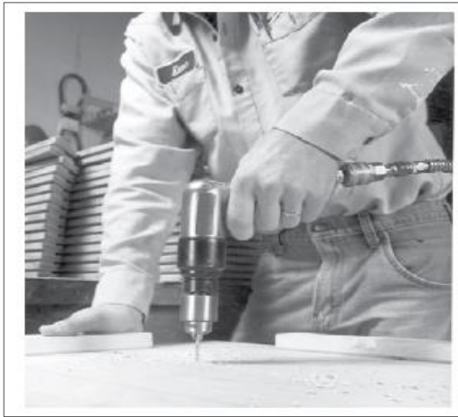
Figure 43 – Operator with portable air drill (CAGI 1998)
