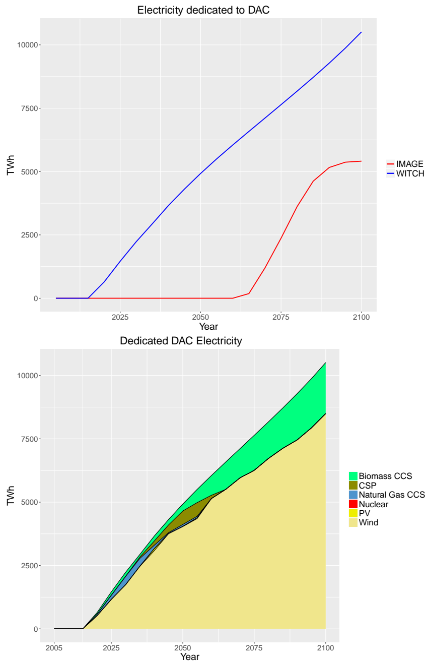
Figure 5.8: World total electricity consumption of DAC in the 1.5°C scenario and the electricity sources powering DAC (WITCH)
