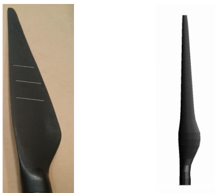
Figure 3.5: Comparison between real and AdWiMo scaled blade
