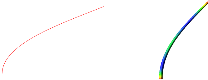
Figure 4.1: First mode of vibration of the tower
