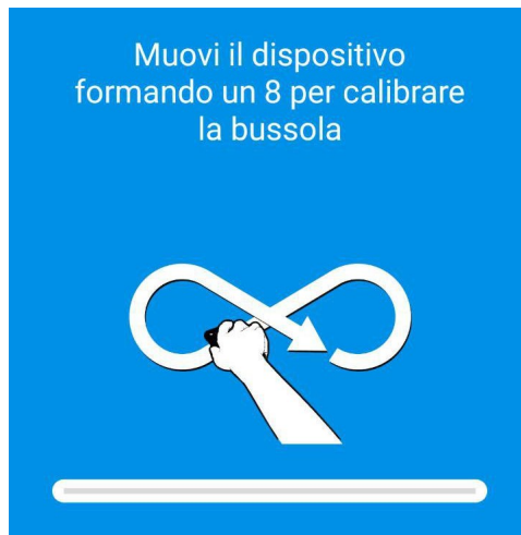
Figure 3.2: Magnetometer Calibration: how to move the device to help the sensor calibration.
