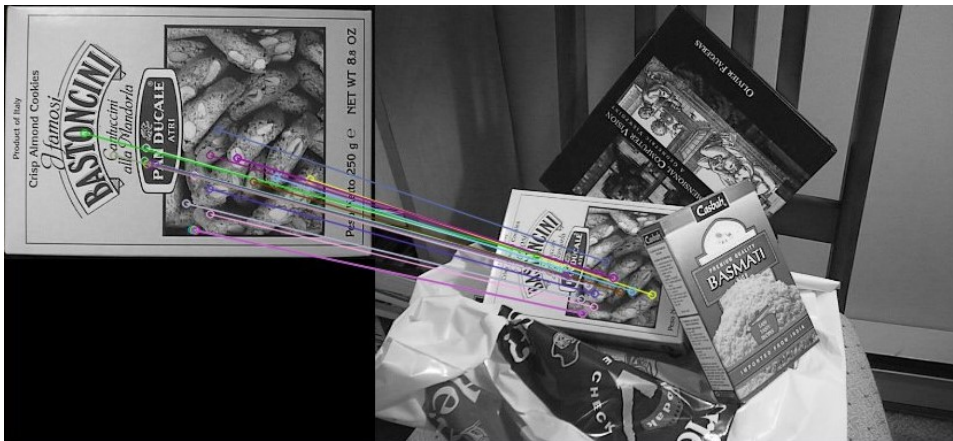
Figure 2.2: An example of the feature-based image registration process.
