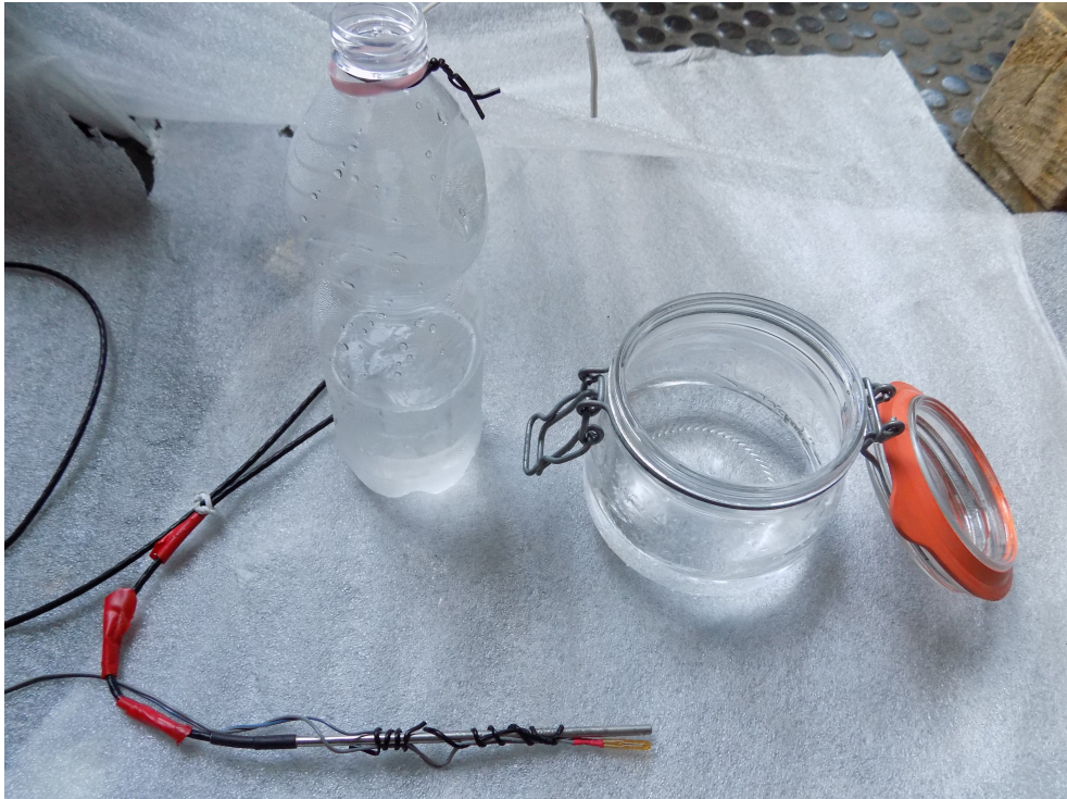
Figure 5.15: First set-up of test for the thermistor calibration: the plastic and rigid container and the two temperature sensors. In the lower part of the figure there are the two sensors: ultra-thin and the heavier steel sensor linked together to be sure that they are measuring the same temperature in the same point.
