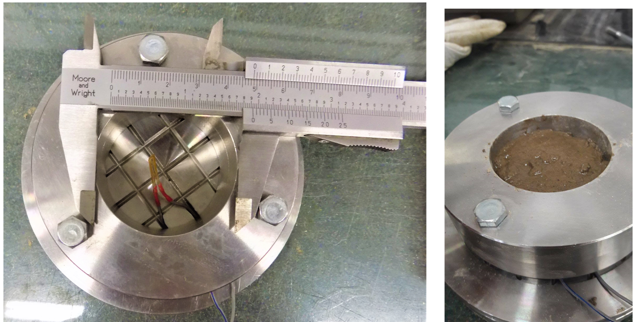
Figure 5.28: Preparation of the soil sample. The temperature sensor is positioned in the end of the mould. Then the mix of soil and water is inserted to cover entirely the sensor. In this way we obtain the temperature data at the soil core.
