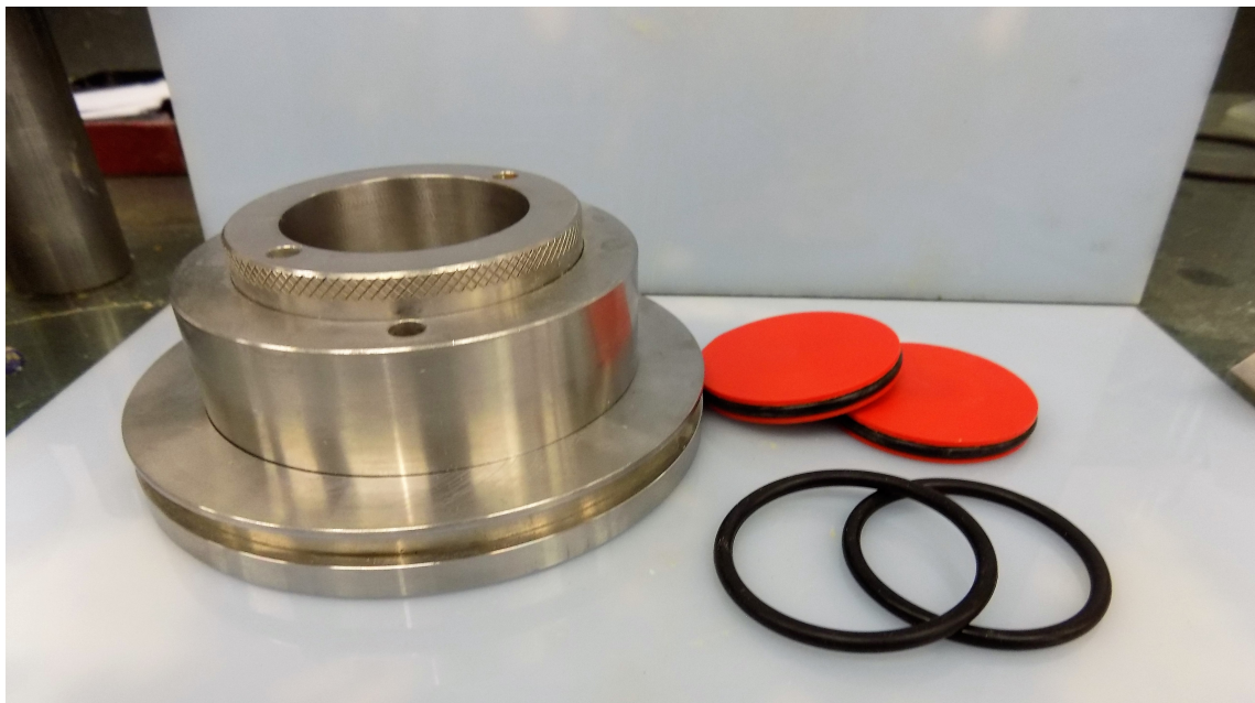
Figure 5.3: Photo of the soil cell elements: on the right two O-Ring and the two plastic discs with the O-ring. On the left the mould utilized.
