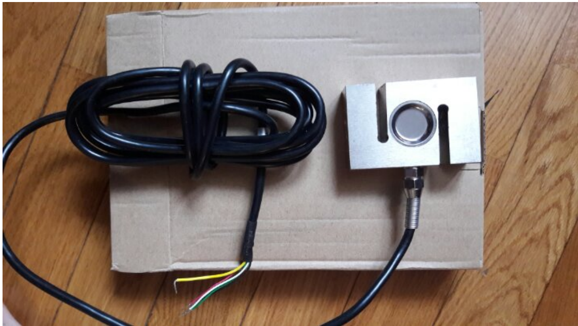
Figure 5.5: load sensor to measure the force.
