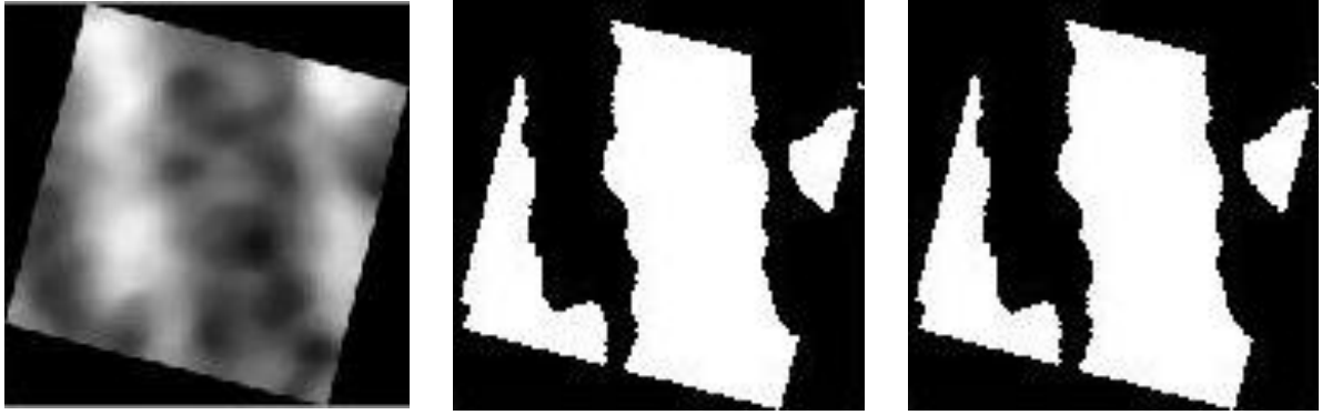
Figure 32 – On the left, original gray scale cropped image. In the middle, cropped binarized image obtained with Otsu's method. On the right, cropped binarized image obtained with kmeans function with k=4 .
