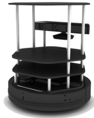
Figure 6.4: TurtleBot equipped with Kinect sensor.
