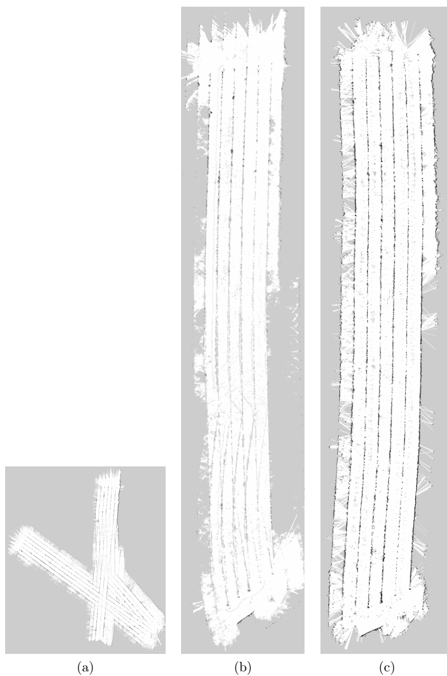
Figura 6.3: Maps of the MasLlunes vineyard built using robot localization. (a) KartoSLAM (Feb), completely wrong, (b) Google's Cartographer (Feb), the map presents some erroneous lines in the lower part, (c) Gmapping (Feb), acceptable map, even if slightly curve, but this usually does not interfere with the localization algorithm
