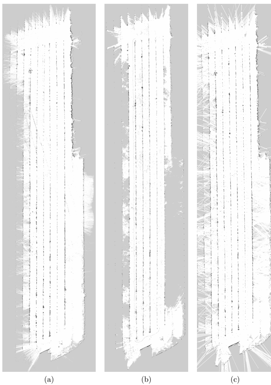
Figura 6.4: Maps of the MasLlunes vineyard built using ROAMFREE. (a) KartoSLAM (Feb), there are some inaccuracies and it is not acceptable without manual cleaning, (b) Google's Cartographer (Feb), it is a perfect map, (c) Gmapping (Feb), it is very good and straight
