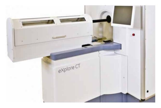
High-resolution X-ray CT is a technology that provides non-destructive three-dimensional mapping of density, enabling topology, structural visualization and quantitative analysis for a wide variety of samples, including live vertebrate and invertebrate animals, insects, plants, fossils, electronics and materials.
