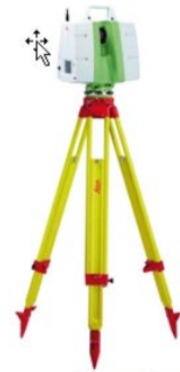
Figure 2.2 Time of Flight Scanner
