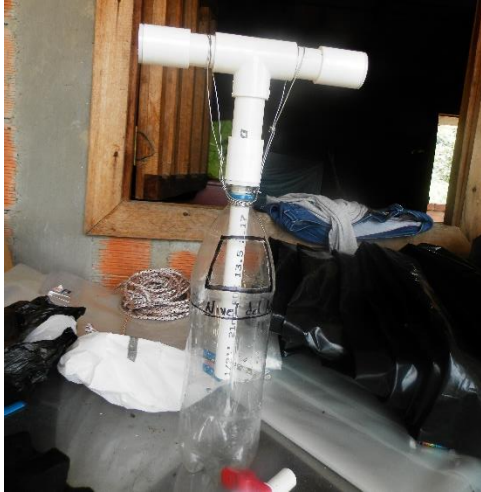
Figure 5.14 Safety valve during the construction phase.
