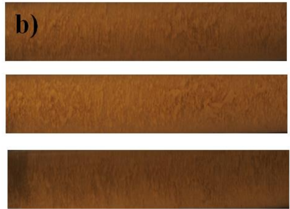
Figure 4-2 Flow pattern for downstream sudden expansion 21-30 mm for J_o=3.35 m/s, a) J_w=2.40 , b) 2.80 m/s
