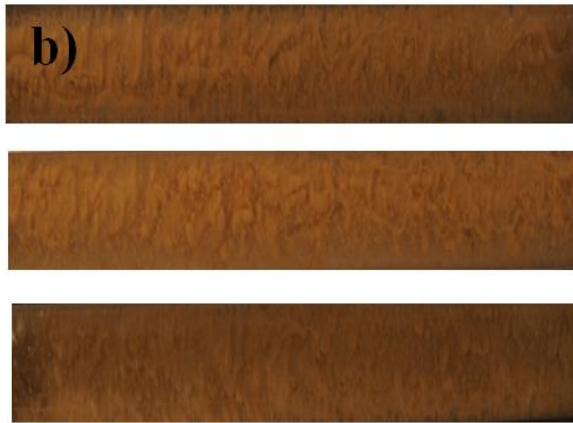
Figure 4-1 Flow pattern for downstream sudden expansion 21-30 mm for J_o=2.23 m/s, a) J_w=2.40 , b) 2.80 m/s
