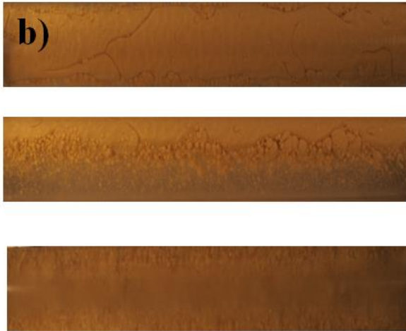
Figure 4-5 Flow pattern for downstream sudden expansion 30-50 mm for J_o=1.09 m/s, a) J_w=1.17 , b) 1.37 m/s
