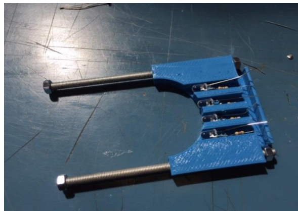
Figure 8-1 Image of 3D printed elements of optical sensor
