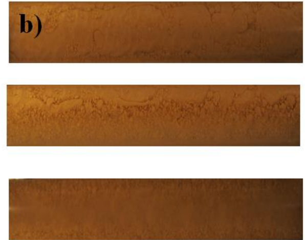
Figure 4-6 Flow pattern for downstream sudden expansion 30-50 mm for J_o=1.64 m/s, a) J_w=1.17 , b) 1.37 m/s
