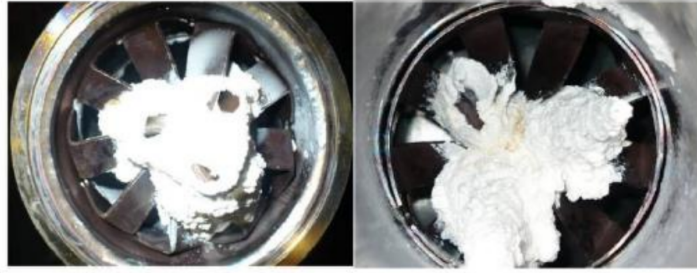
Figure 1.5: Urea by-product deposits on a static mixer [62].
