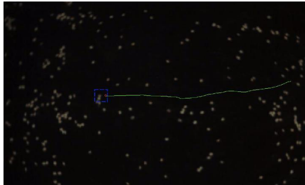
Figure 4.3. Example of partially tracked particle, mismatch due to the presence of several particles in the search window (blue rectangular represents the search window).
