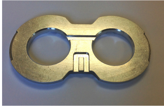
Figure 1.2: Decompression slots in the compensation plates of a gear pump [27]
