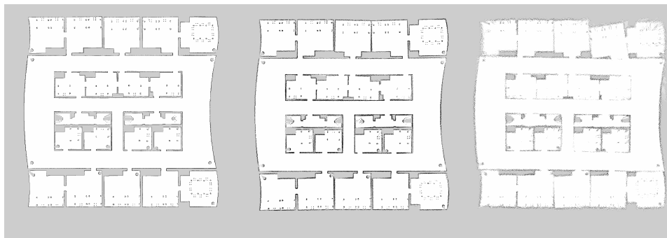
Figure 6.7: The leftmost map is built without noise, the central map with 0.1 Gaussian noise, and the rightmost one with 0.3 Gaussian noise.
