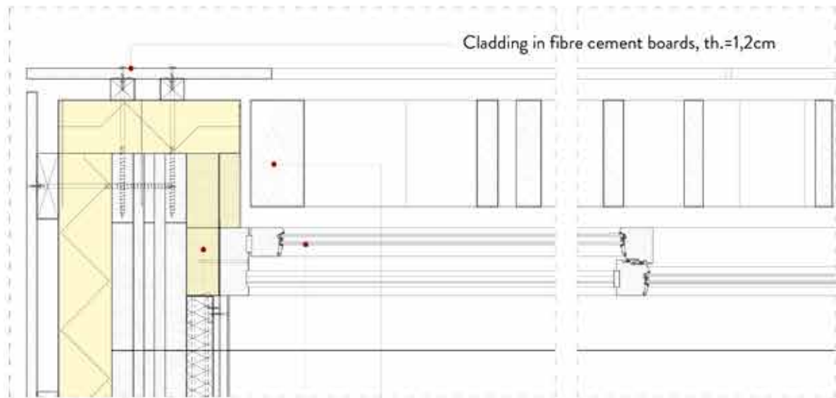
Board 4.18 Horizontal section of half unit (module with Voronoi screen and door)
