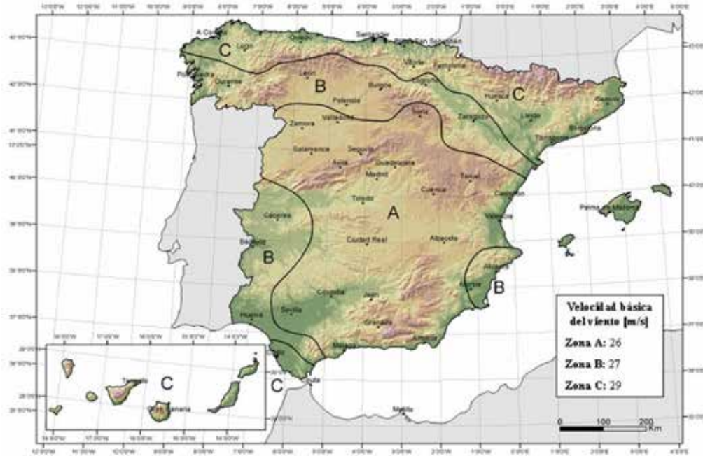
Figure 4.58 Fundamental value of the basic wind velocity
