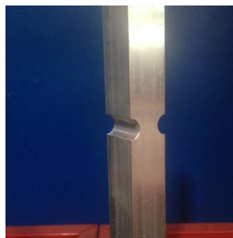
Figure 52 Notched bar used in the experimental activity
