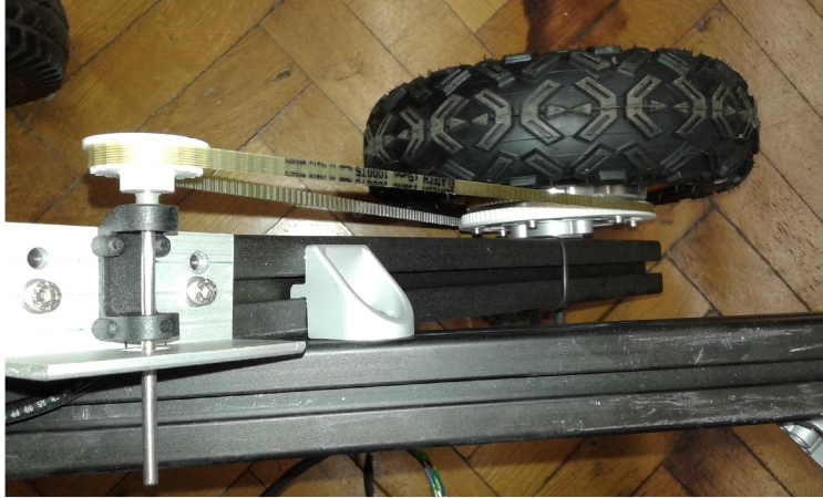
Figure 4.2: Encoder transmission configuration
