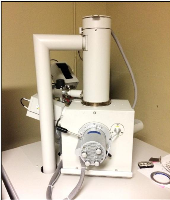
Scanning electron microscopy (SEM) were performed in order to obtain high resolution images, referring to the superficial textures of the samples; a FEI Quanta 250 microscope (Figure 4.3, ThermoFisher Scientific, Hillsboro, USA) operating in low-vacuum modality was used.
