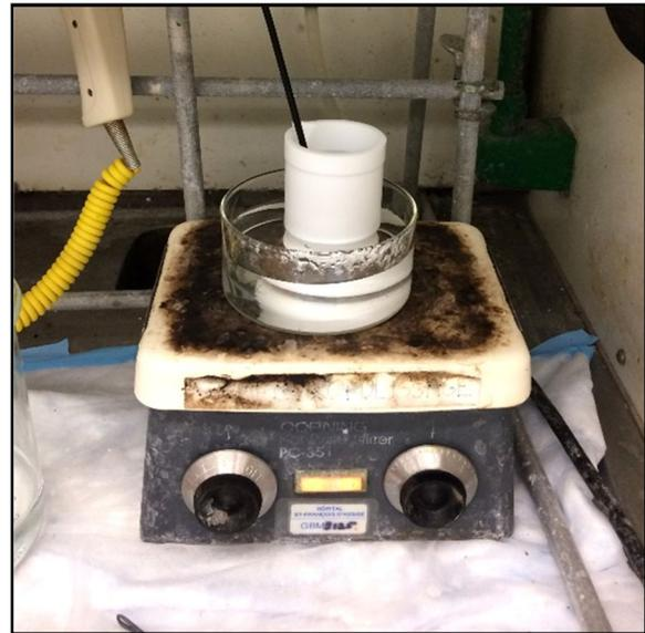
Figure 4.1: (A) Glycerol-based bath and (B) hydrofluoric acid-based solution for electropolishing process (Laboratory of biomaterials and bioengineering (LBB), Quebec City, Canada)
