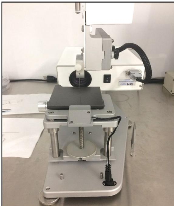
Static contact angle measurements were performed to evaluate the wettability of treated surfaces. In this regard, a video contact angle system (Figure 4.4, AST Products Inc. VCA 2500 XE, Billerica, USA) was used. The analysis was carried out in different parts of the same sample, at r.t. and using 1  $\mu$ L droplets of double deionized water, deposited by means of a syringe.
