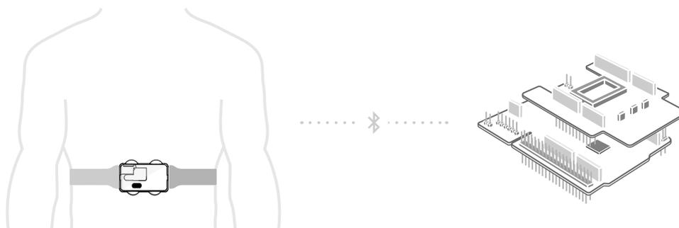
Figura 1: The Bio2Bit device acquires and transmits in real-time the ECG trace to the NUCLEO STM32 board.
