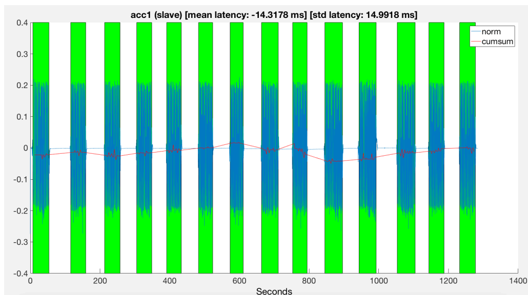
Figure 3.9: Experimental validation session. The bar is rolled back and forth various times within 14 intervals spaced apart. The red line represents the progress of the relative cumulative delay between one accelerometer (slave) and one OpenBCI (master).
