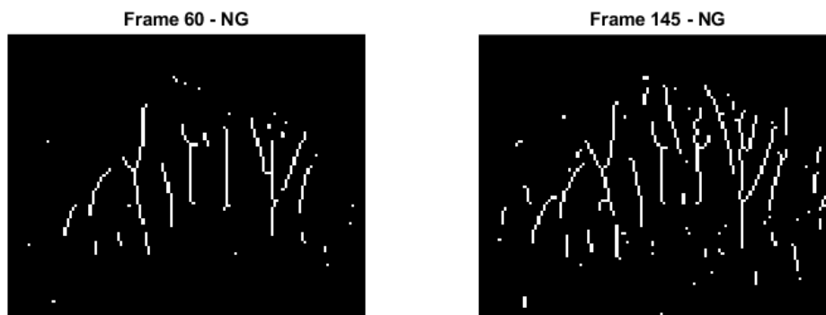
Figure 4.32: Example of NG image skeletons: left skeleton is taken from a baseline frame, while right one from a frame after NG injection.
