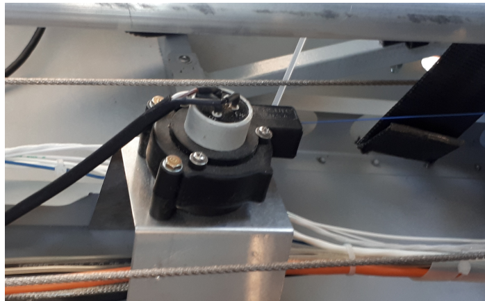
Figure 3.2: One of the potentiometers installed on the G70 TRAIL.
