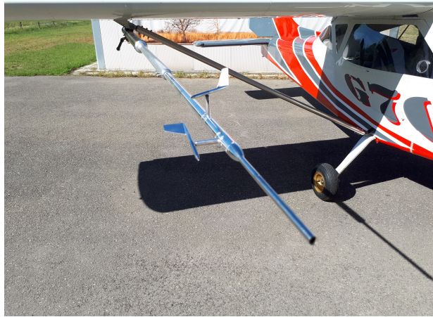
Figure 3.4: The air data boom.
