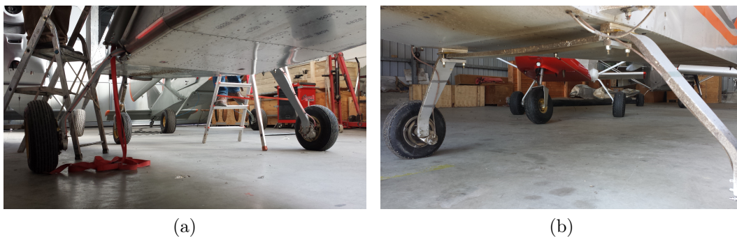
Figure 2.6: The new (2.6a) and the old (2.6b) landing gear.
