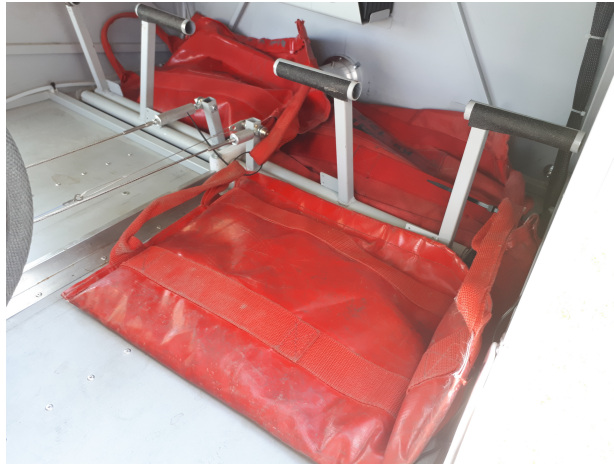
Figure 6.4: Ballasts position to achieve full forward CG, during flight 04.1706.
