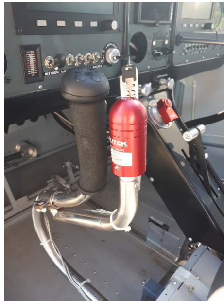
Figure 3.5: The instrumented stick bar, with the stick force sensor.
