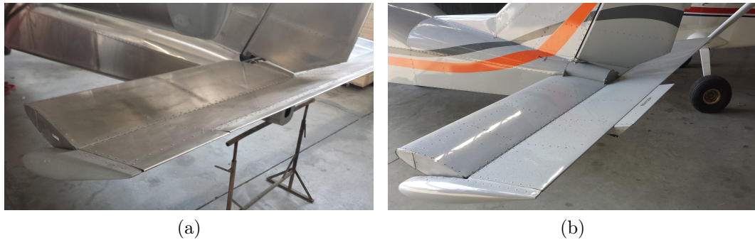
Figure 2.4: The new (2.4a) and the old (2.4b) elevator and trim tab.
