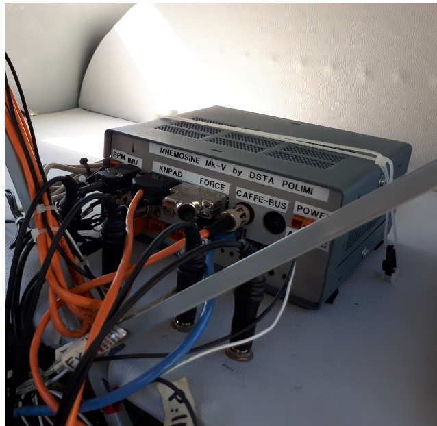
Figure 3.1: Mnemosine main unit, housed in the luggage compartment behind the seats.
