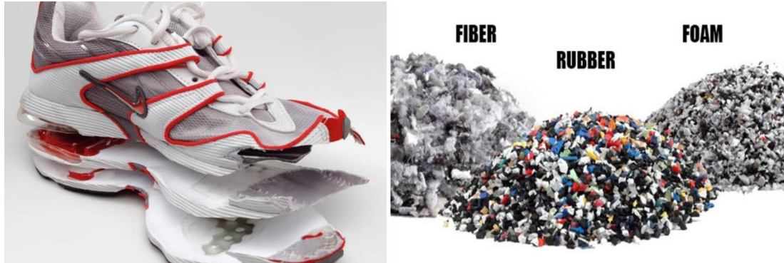
Figure 1. 6 - NIKE shoes taken apart into 3 parts
