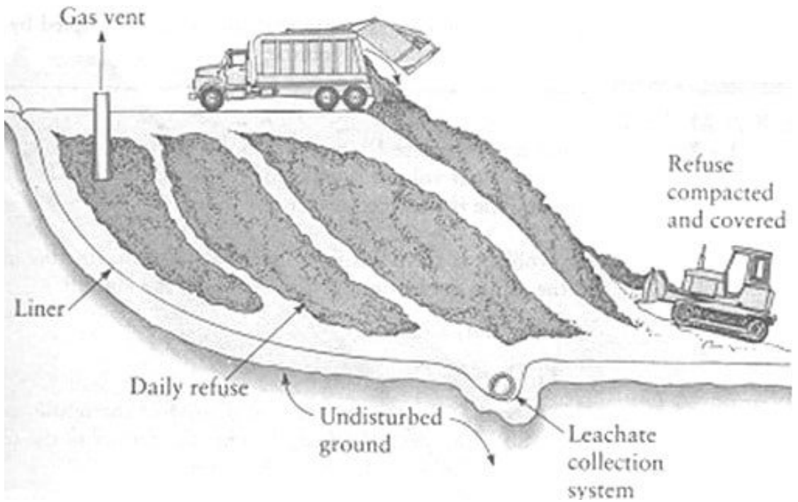
Figure 1.11 "Landfill" process
